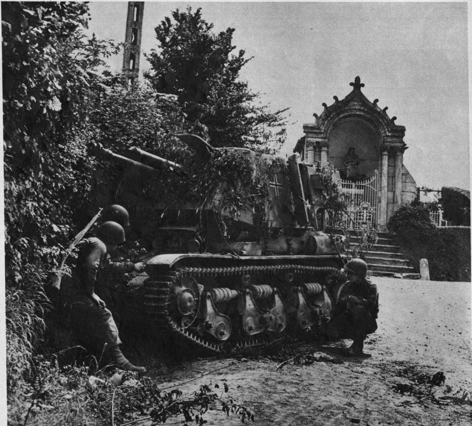
Hotchkiss 39 tank with a captured Czech 47-mm. gun is another instance of Nazi-used French equipment. German ingenuity salvaged the
